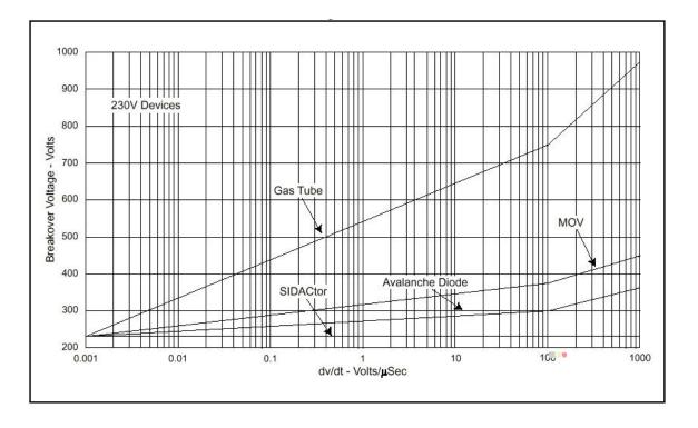
From viewing the chart, the Sidactor's breakover voltage level was unchanged over varying rise times. The gas tube had a substantial increase in breakover performance as the rise time increased. The sub par performance of the gas tube over increased rise times would allow significant amounts of let thru voltage into the protected equipment, whereas a Sidactor maintains a consistent performance over increasing rise times.
