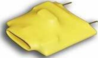
Amplifier manufacturers and aftermarket manufacturers of replacement amplifier modules are offering plug in surge protectors to protect amplifiers. The units consist of a plug in crowbar surge protector. A crowbar device consists of 2 SCRS and a diode to trigger the device. The device senses an overvoltage and shunts it to ground, much like a Sidactor. These units are offered by the amplifier manufacturers as a solution to damage to the amplifier circuitry caused by surges.
